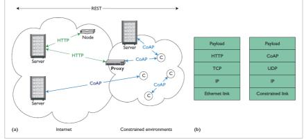
Implementing the Web architecture with HTTP and the Constrained Application Protocol (CoAP). (a) HTTP and CoAP work together across constrained and traditional Internet environments; (b) the CoAP protocol stack is similar to, but less complex than, the HTTP protocol stack.
