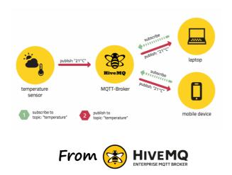
Decoupled in space and time. The clients do not need each other's IP address and port (space) and They do not need to be running at the same time (time).
