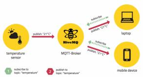
In the picture, replace the laptop with an actuator, subscribing to a command topic, say, device3/commands. Replace the sensor with a browser ending commands to device3/commands.
