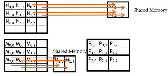
Threads (1,0) and (1,1) need special treatment in loading M tile
